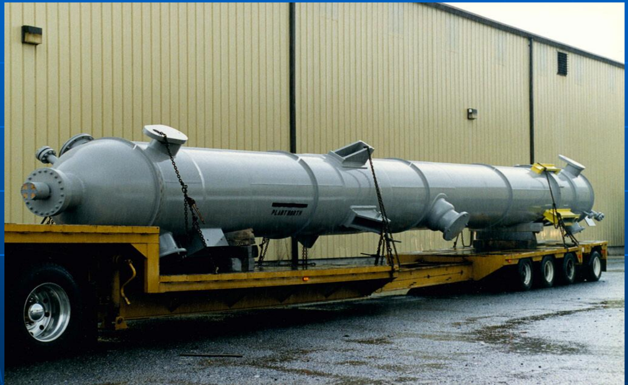
Liquefied Natural Gas (LNG) Regasification Vaporizer
